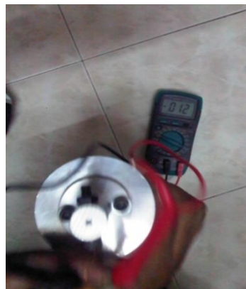
Figure 5 Voltage recording using multimeter
