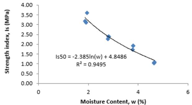
**Figure 6** Reduction in strength index due to moisture content increase for Grade III sandstone
