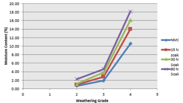
**Figure 4** Pattern of water absorption with different stage of weathering
