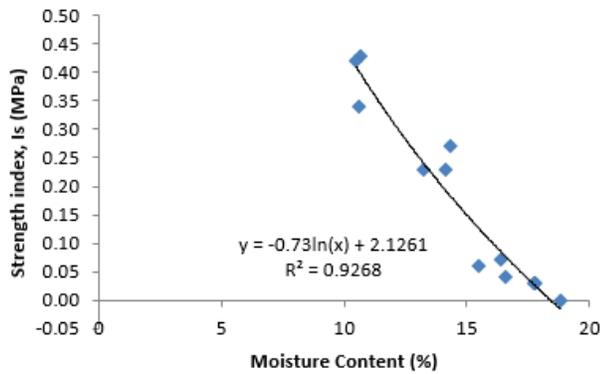
**Figure 7** Reduction in strength index due to moisture content increase for grade IV sandstone
