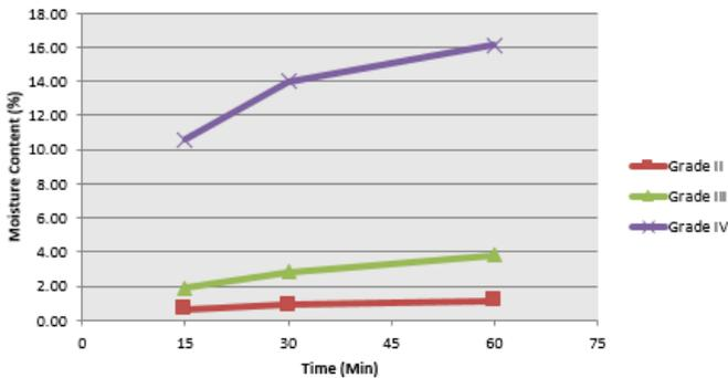
**Figure 3** Variation in the absorption of moisture content with time for different weathering grade
