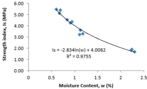
**Figure 5** Reduction in strength index due to moisture content increase for Grade II sandstone
