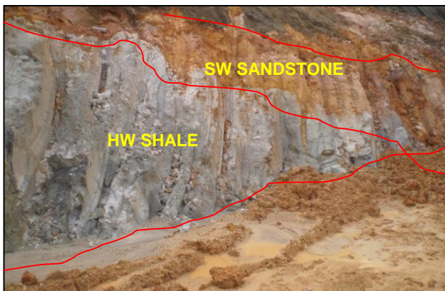
Figure 2 Geological model of weak shale with strong sandstone
