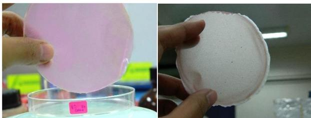
**Figure 2** (a) Film from PSP and (b) Film from SP added with BHA
