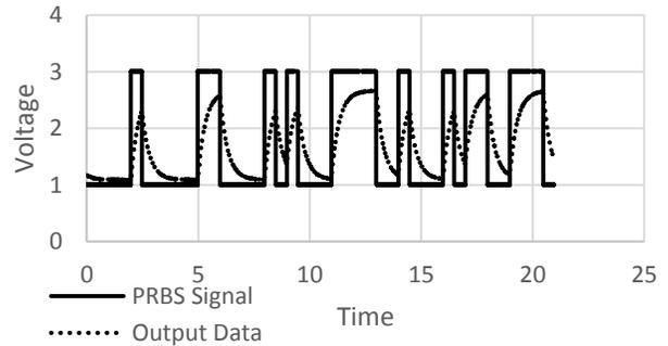
**Figure 5** Data collected for system identification process using modulo 6 & 7
