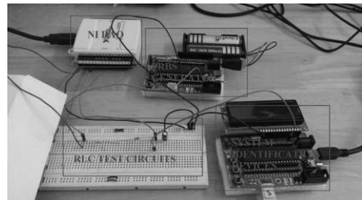
Figure 3 System identification microcontroller platform
