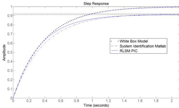
Figure 6 Step response for both system identification result
