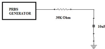
**Figure 4** RC circuit
