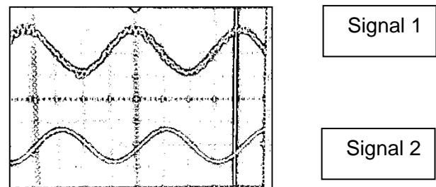
**Figure 4** Output signal from detection electrode (signal 1) and AC capacitance measuring circuit (signal 2)
