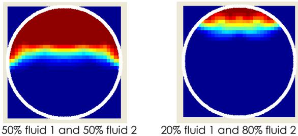
**Figure 5** Cross-section image of mixing fluids inside the pipeline
