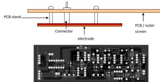
Figure 2 Electrode mounted together with guard and receiving circuit
