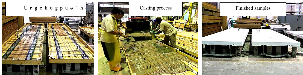
Figure 2 Full-scale test specimens preparation
