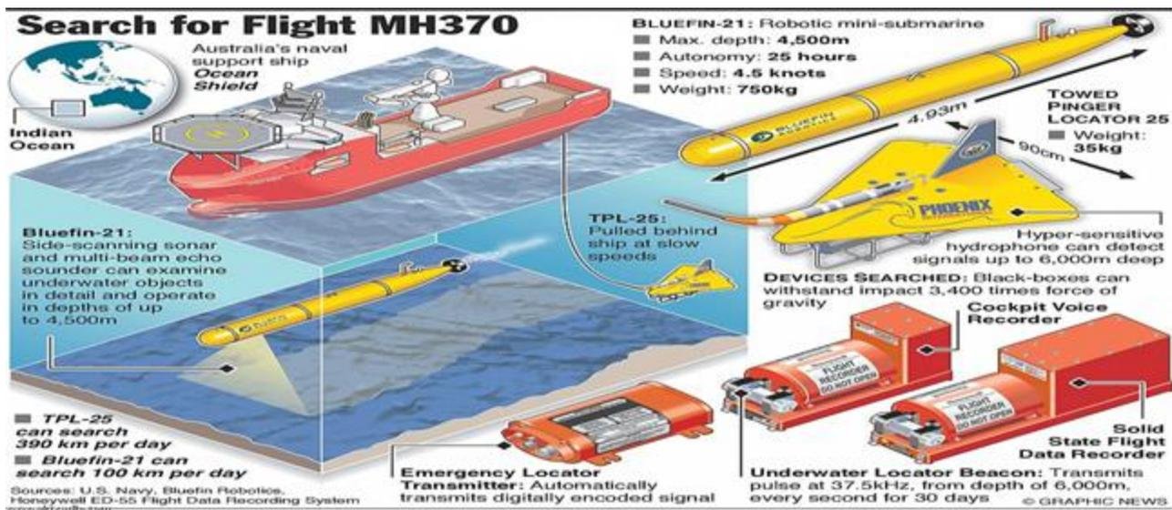
Figure 4 Ocean shield, towed pinger locator and Bluefin-21 Sonar system
