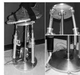
Figure 2 2-DOF parallel robot
