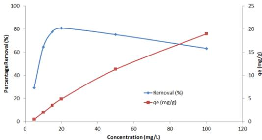
Figure 2 Effect of initial BPA concentration onto durian peel
