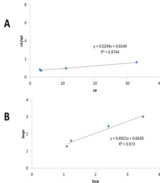
Figure 4 Langmuir model (A) and Freundlich model (B) for adsorption of BPA onto durian peel
