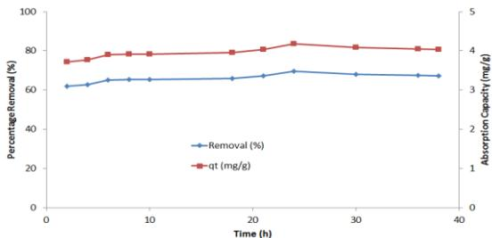
Figure 3 Effect of contact time on BPA adsorption by durian peel
