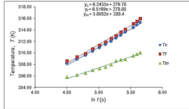
Figure 4 Graph of temperature variations of the three samples; dry coarse sand ( $T_c$ ), dry fine-medium sand ( $T_f$ ) and MgO powder ( $T_m$ ) versus natural log of time ( $\ln t$ ).  $y_c$ ,  $y_f$  and  $y_m$  are the respective trend line linear equations for  $T_c$ ,  $T_f$  and  $T_m$
