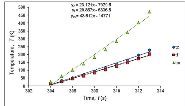
Figure 5 Graph of temperature ( $T$ ) versus time taken to attain temperature for dry coarse sand ( $t_c$ ), dry fine-medium sand ( $t_f$ ) and MgO powder ( $t_m$ ).  $y_c$ ,  $y_f$  and  $y_m$  are the respective trend line linear equations for  $t_c$ ,  $t_f$  and  $t_m$
