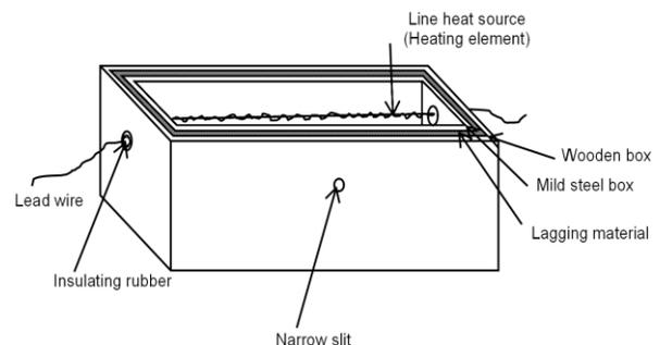
**Figure 1** Schematic diagram of the electric heating equipment
