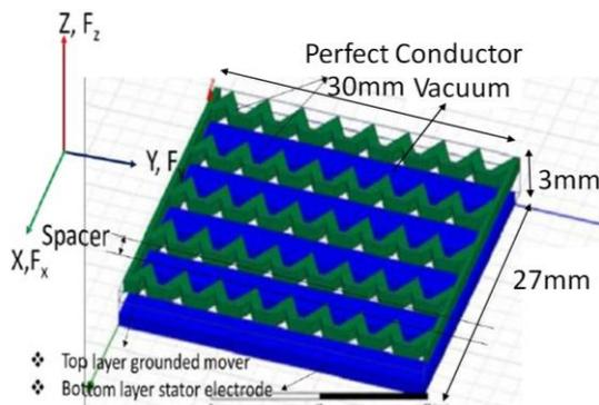
(b) Skew-Type Electrostatic Motor
