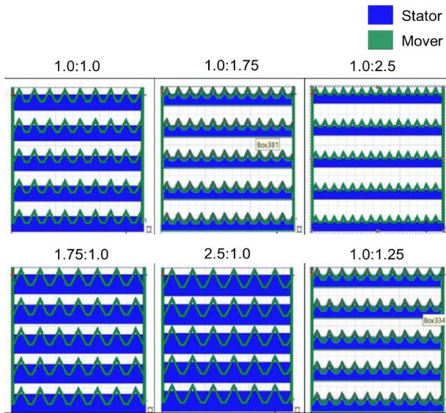
**Figure 3** Structure of the skew-type electrostatic motor when the electrode: spacer ratio is varied
