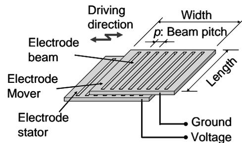
(a) General schematic of the electrostatic motor
