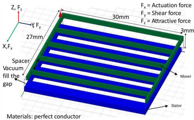
(a) Non-Skew-Type Electrostatic Motor
