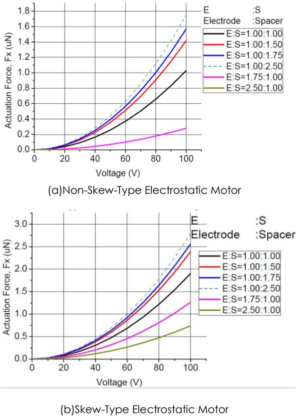
**Figure 4** Comparison of the generated thrust force between the two designs when the Electrode: Spacer ratio is varied and evaluated with different input voltages
