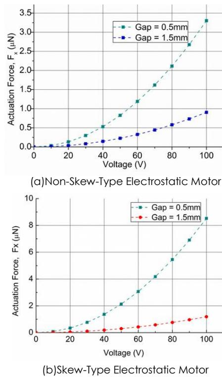
**Figure 5** Comparison of the generated thrust force between the two designs when the gap is varied, evaluated with different input voltages
