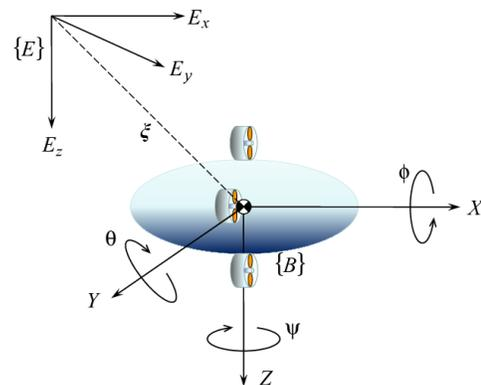
Figure 1 Coordinate systems of AUV
