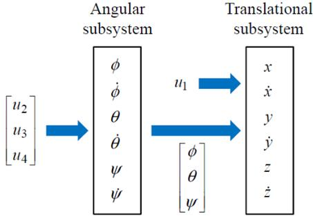
**Figure 2** Connection of rotational and translational subsystems
