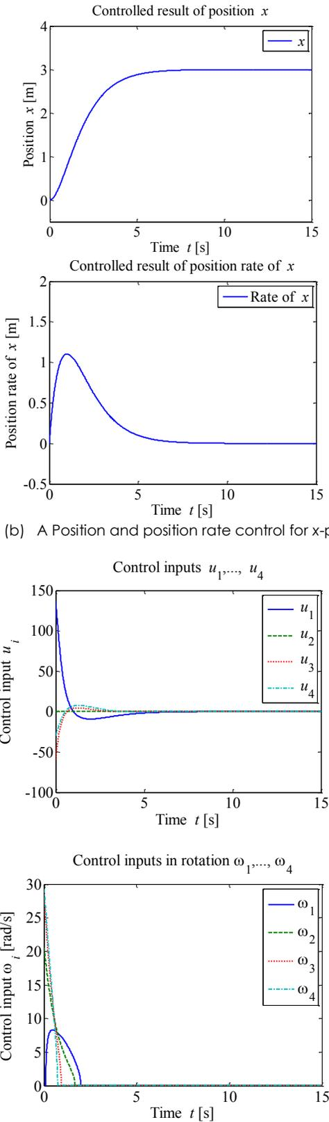
(b) A Position and position rate control for x-position
