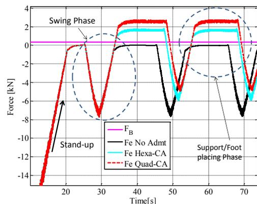
**Figure 7** Sample of vertical force on foot for both Sim 1 and 2 (sample: Leg 3)
