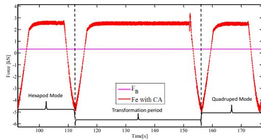
**Figure 8** Sample of vertical force on foot in Sim 3 (sample: Leg 1)
