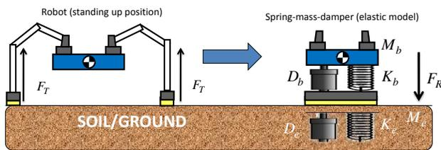
Figure 2 Equivalent elastic model of the robot's body
