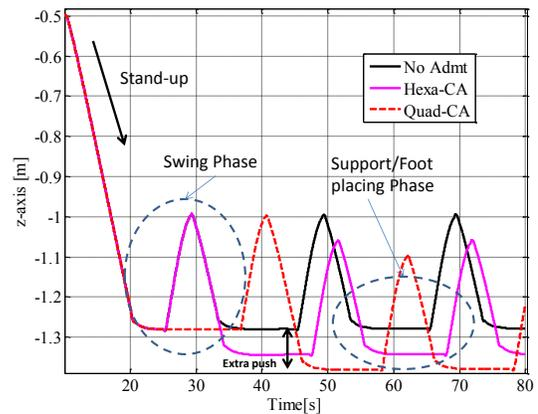
**Figure 6** Sample of foot point motion on the z-axis output for both Sim 1 and 2 (sample: Leg 3)
