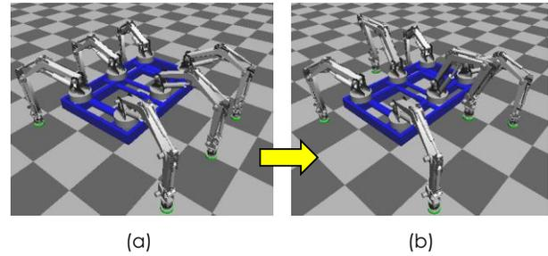
Figure 4 CLD transformation in proposed hexa-quad transformation: (a) hexapod mode, and (b) quadruped mode
