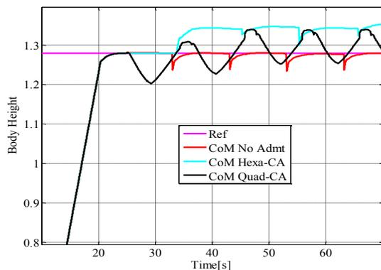
**Figure 10** Sample of CoM signal representing robot height performance
