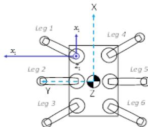
Figure 3 Coordinate system and leg's notification for hexapod robot model
