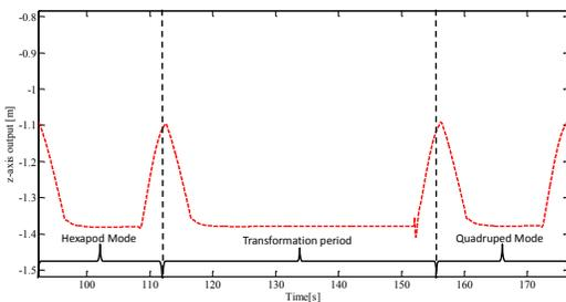
**Figure 9** Sample of foot point motion on the z-axis output for Sim 3 (sample: Leg 1)
