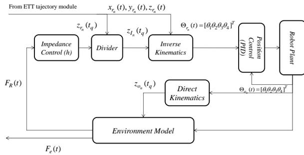
**Figure 5** Implementation of the proposed CoM-based admittance control on the 4-DoF leg configuration hexapod robot model
