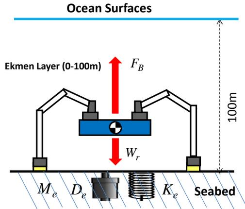
**Figure 1** Buoyant force acting on multi-legged robot in underwater
