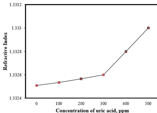
**Figure 5** The measured refractive index at different concentrations of uric acid
