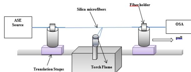
**Figure 1** Schematic diagram of the tapering process of the SOF using flame brushing technique
