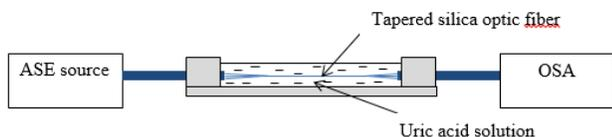
**Figure 3** The experimental setup for the proposed sensor to detect different concentrations of uric acid using a tapered SOF coated with ZnO nanostructures
