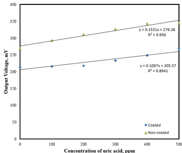
**Figure 4** Output voltage against uric acid concentrations for the fabricated tapered SOF coated with ZnO and non-coated
