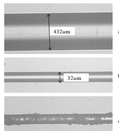
**Figure 2** Shows the microscope images of SOF with (a) original fiber, (b) tapered SOF and (c) tapered SOF coated with ZnO
