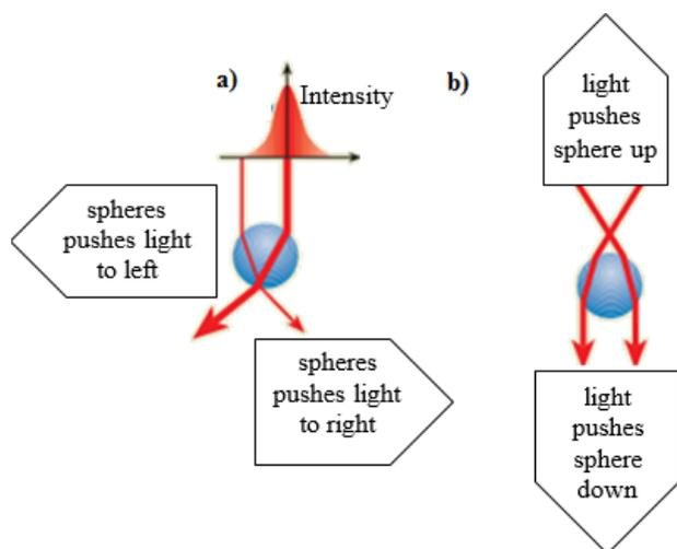
Figure 1 Rays pathway of the laser beam
