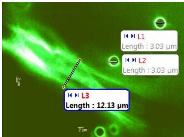
**Figure 2** Polystyrene beads (circular shape) in nanocellulose solution, fibrous structure can be seen
