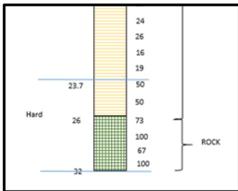
Figure 7 Details of BH13 bore log
