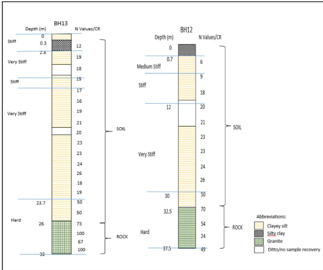
Figure 6 Details of rock cores of BH13 and BH12
