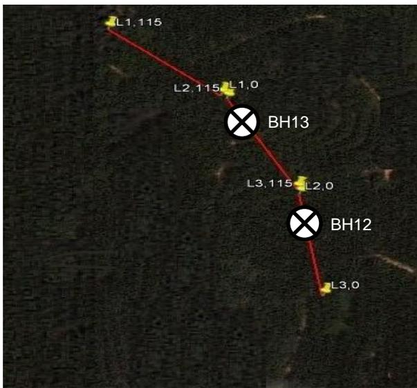
Figure 4 Location of survey lines for seismic refraction (red) and existing borehole (white)
