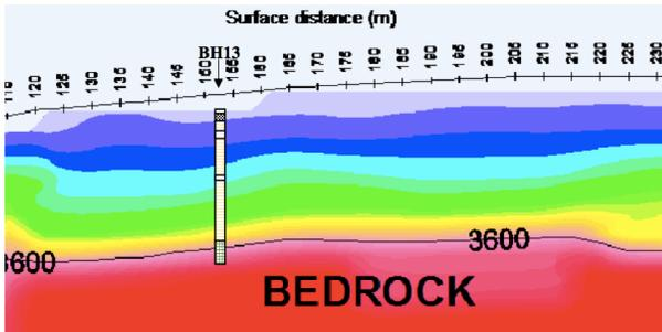
**Figure 8** The combination of seismic section (L2) and BH13 in Ulu Tiram
