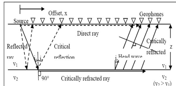
**Figure 1** Ray path diagram showing the respective paths for direct, reflected and refracted rays [3]
