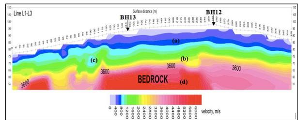
Figure 5 Seismic section of velocity gradient at L1-L3 survey line in Ulu Tiram (Johor)
