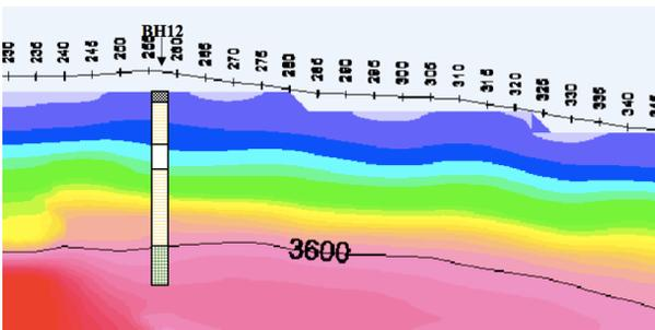
**Figure 9** The combination of seismic section (L3) and BH12 in Ulu Tiram
