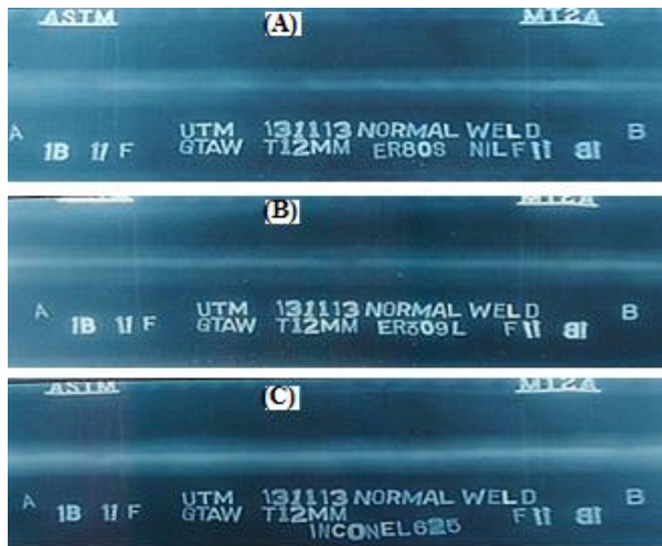
Figure 2 Radiography results of welds of (A) 80S-Ni1 (B) 309L (C) Inconel 625
