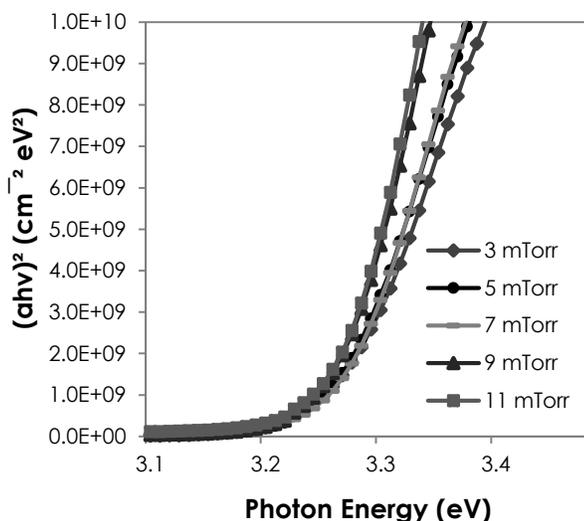
**Figure 5** Plot of graph  $(\alpha h\nu)^2$  versus photon energy for ZnO films deposited on plastic substrate at different sputtering pressure
