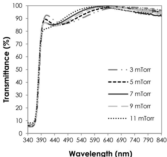
**Figure 4** Optical transmittance spectra of ZnO films deposited on plastic substrate at different sputtering pressure
