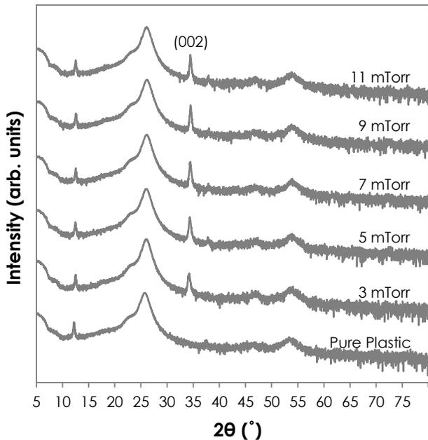
Figure 2 X-ray diffraction patterns of investigated ZnO films deposited on plastic substrate at different sputtering pressure
