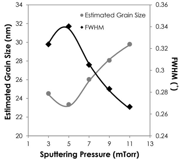
Figure 3 The variation of full width at half maximum (FWHM) and estimated grain size of ZnO (002) diffraction peak at different sputtering pressure
