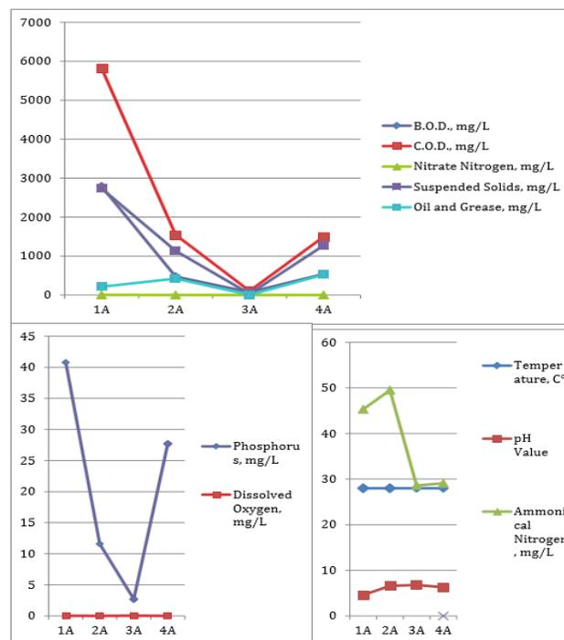
**Figure 1** Measured BOD, COD, oil & grease, suspended solids and nitrate nitrogen
