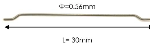
Figure 1 Geometry of steel fibre
