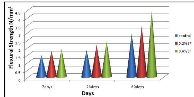
**Figure 8** The comparison of flexural strength of control sample with steel fibre reinforced foamed concrete of 1200 kg/m<sup>3</sup> density
