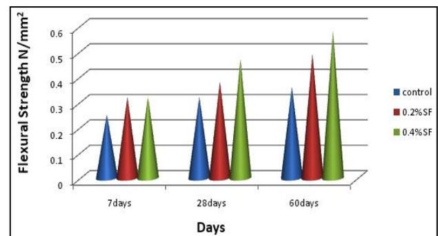
**Figure 8** The comparison of flexural strength of control sample with steel fibre reinforced foamed concrete of 700 kg/m<sup>3</sup> density
