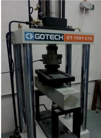
Figure 3 Setup for bending test
