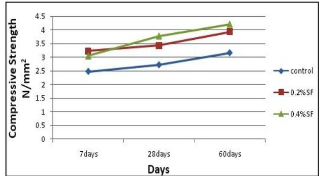
Figure 5 The comparison of compressive strength of control sample with steel fibre reinforced foamed concrete of 1200 kg/m<sup>3</sup> density
