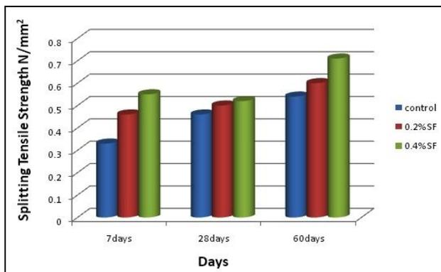
**Figure 7** The comparison of splitting tensile strength of control sample with steel fibre reinforced foamed concrete of 1200 kg/m<sup>3</sup> density
