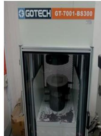
Figure 1 Apparatus for compression test
