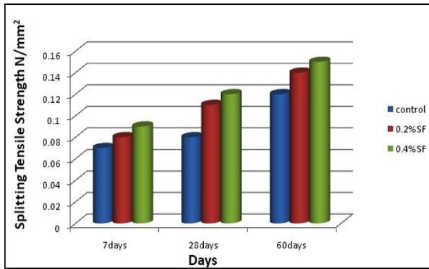
**Figure 6** The comparison of splitting tensile strength of control sample with steel fibre reinforced foamed concrete of 700 kg/m<sup>3</sup> density
