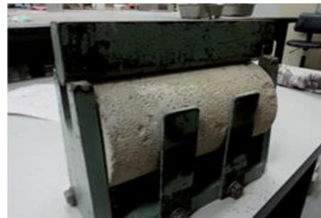
Figure 2 Setup for splitting tensile test
