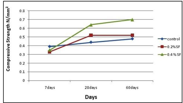
Figure 4 The comparison of compressive strength of control sample with steel fibre reinforced foamed concrete of 700 kg/m<sup>3</sup> density
