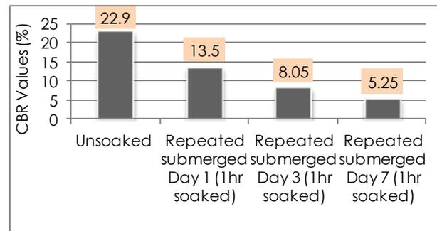
**Figure 5** Comparison of CBR values between unsoaked sample and repeated submerged samples
