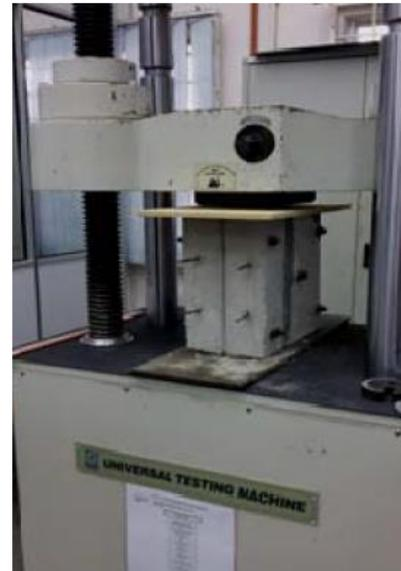
**Figure 2** The Universal testing machine
