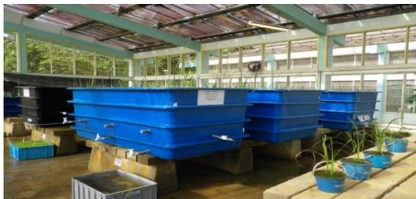
**Figure 3** A pilot scale reed bed with sub- surface flow system
