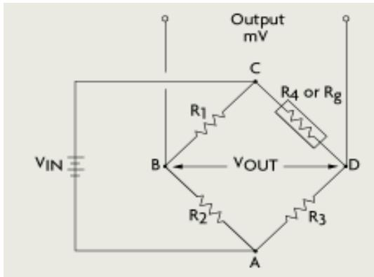
Figure 3 Wheatstone bridge circuit
