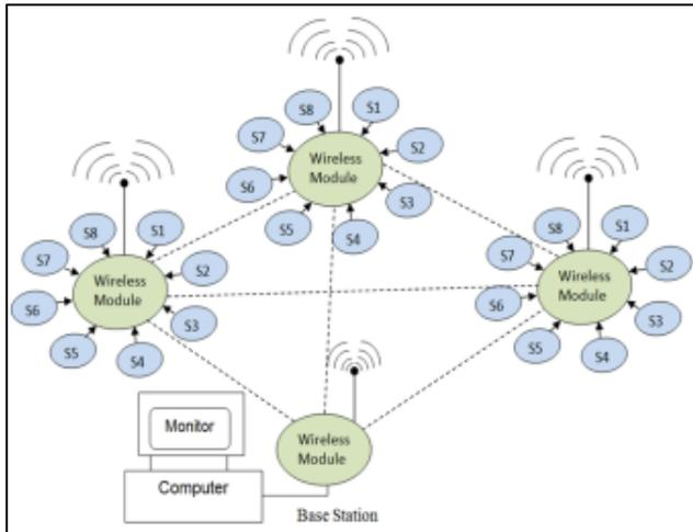
Figure 6 Mesh network using X-Bee-Pro 900HP
