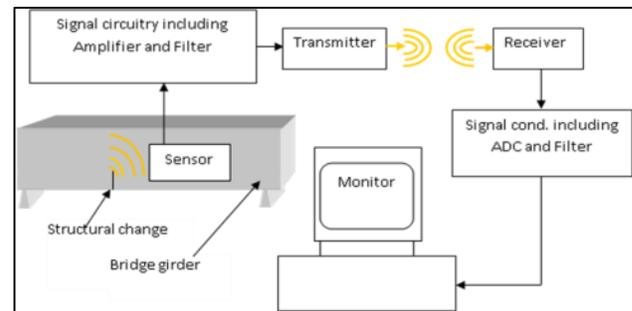
**Figure 2** Block diagram of wireless application on structural health monitoring system
