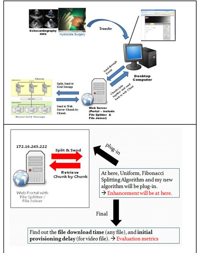
Figure 2 Our grid-based medical video file storage test bed
