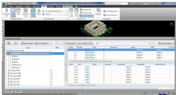
Figure 11 Showing the total quantity takeoff from block partitions in Naviswork Manage 2014
