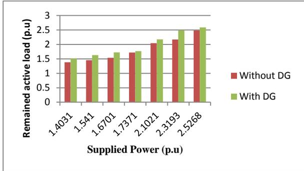
Figure 3 Supplied power (Vs) Remained active load for Test system-1 using IHSA
