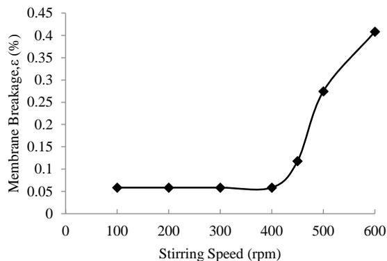
Figure 9 Effect of stirring speed on membrane breakage
