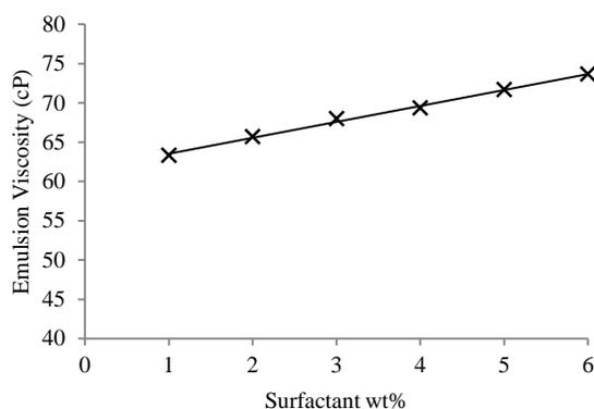
**Figure 4** Plot of emulsion viscosity against surfactant concentration
