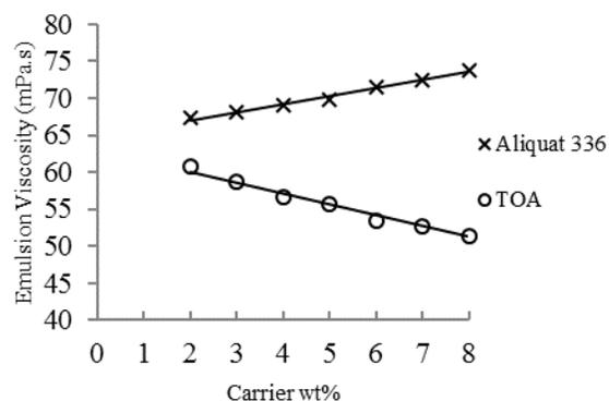
**Figure 2** Plot of emulsion viscosity against carrier concentration
