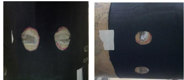
Figure 8 Internal flaws simulated on the pipe surface
