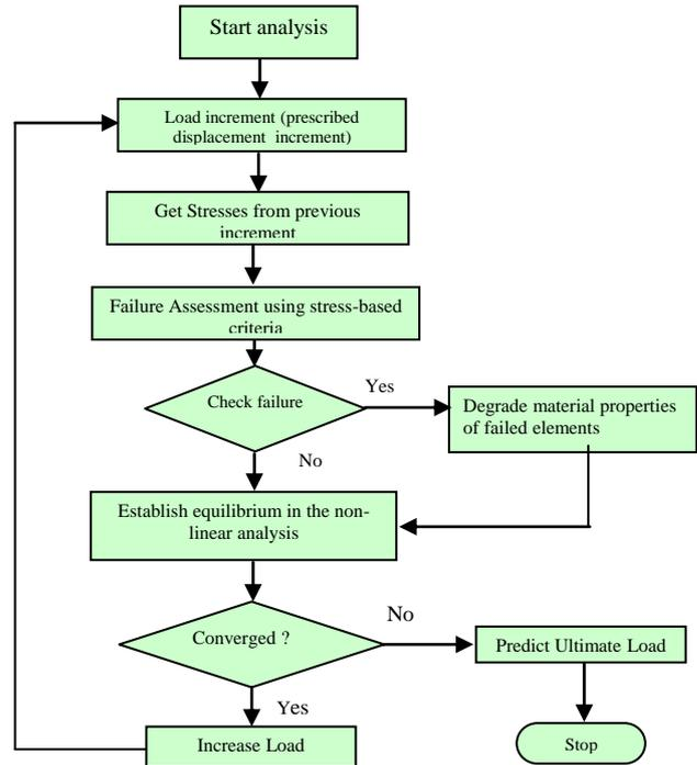
Figure 14 Progressive damage algorithm
