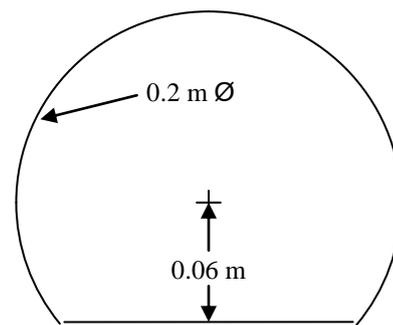
Figure 2: Dimension of the fuselage section
