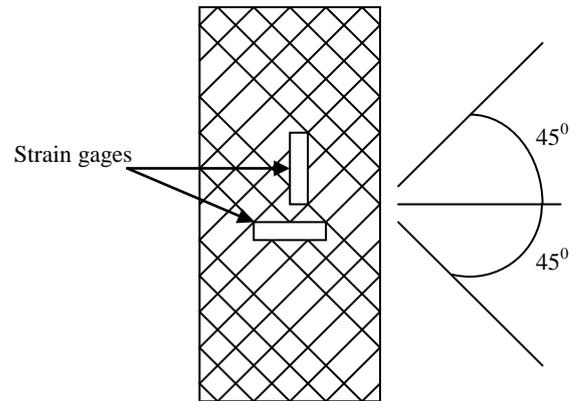
Figure 13: Schematic of a  $[45/-45]_{2s}$  laminate shear test
