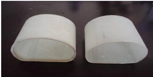
Figure 6: The cured composite fuselage section of type 200g/m<sup>2</sup>
