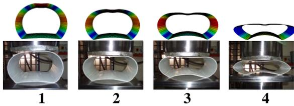
Figure 19: Comparison of deformation photos between simulation and experiment
