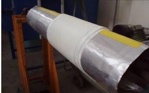
Figure 5: C-glass/epoxy cloth wrapped around the mandrel
