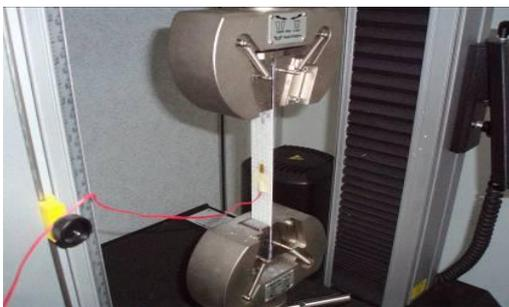
Figure 11: Specimen in the grip of UTM machine
