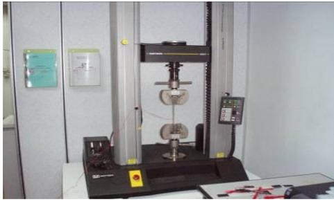
Figure 9: UTM machine for tensile testing
