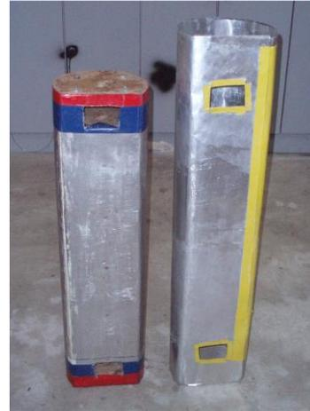
Figure 1: The mandrel and the aluminum outer cover
