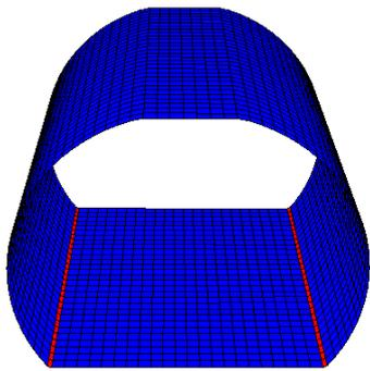
Figure 16 Mesh of the deformable fuselage section
