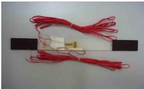
Figure 10: Specimen with the mounted longitudinal and transverse strain gages
