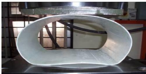
Figure 7: Quasi-static testing using MTS machine
