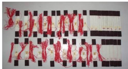
Figure 8: Coupon specimens for tensile testing
