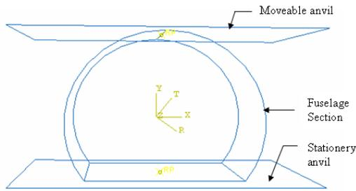
Figure 15: Schematic drawing of the fuselage and boundary conditions
