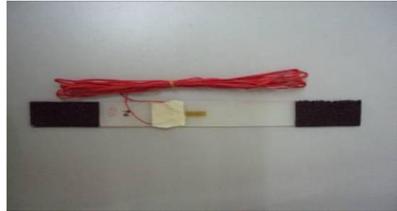
Figure 12: Coupon specimen for determining the transverse tensile property
