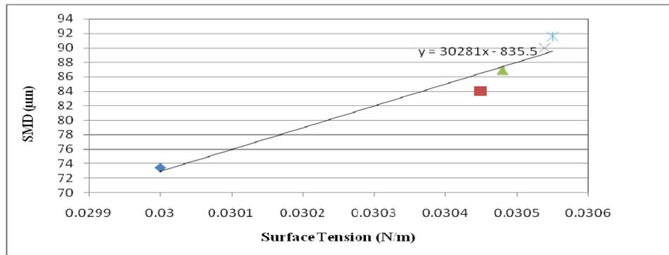
Figure 20: Graph of SMD versus surface tension
