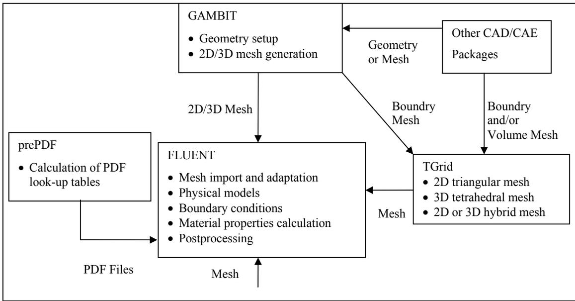
Figure 3: Basic FLUENT Program Structure (FLUENT Modeling & Tutorial Guide)
