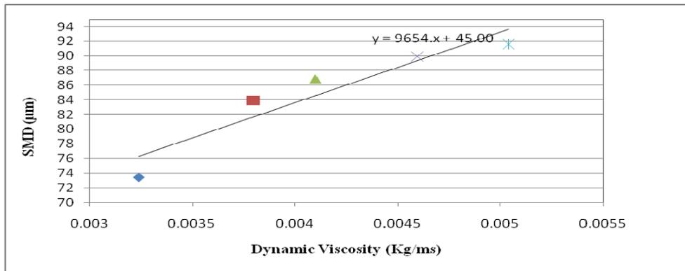
Figure 19: Graph of SMD versus viscosity
