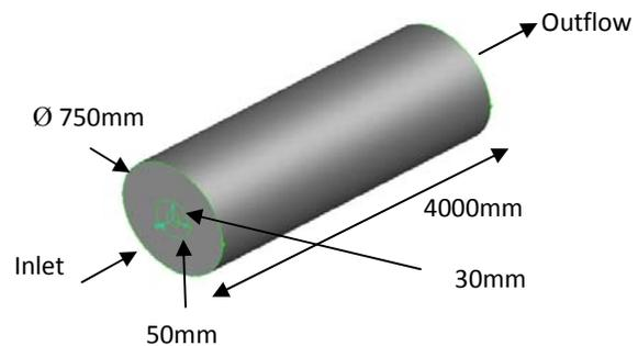
Figure 1: Combustor Geometry
