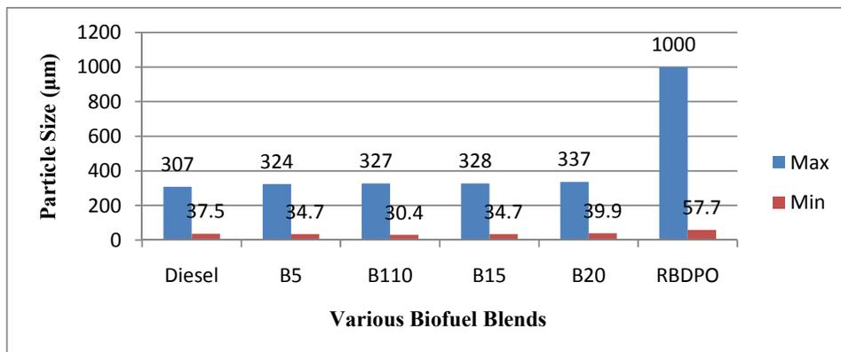
Figure 4: Particle size versus various different fuels
