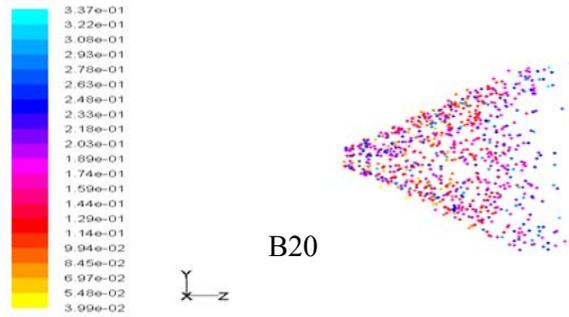
Figure 9: Particle diameter of B20
