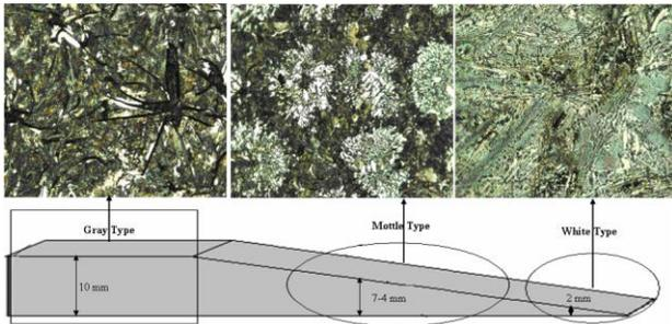
Figure 4 Microstructure of cast iron in various thicknesses; gray type (10 mm), mottle type (4-7 mm) and white type (2 mm)
