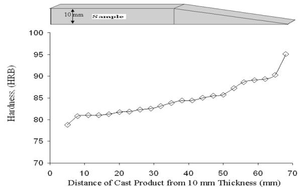
Figure 5 Hardness of the casting from 10 mm to 2 mm thickness in 70 mm length, indentation was made after 2 mm distance
