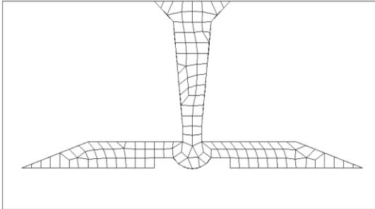
Figure 1 Pattern loaded in FEA software for analysis of sand mould
