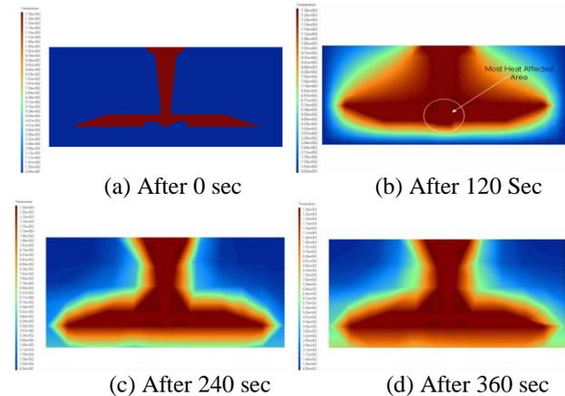
Figure 2 Simulation of temperature distribution on the sand mould using FEA software.
