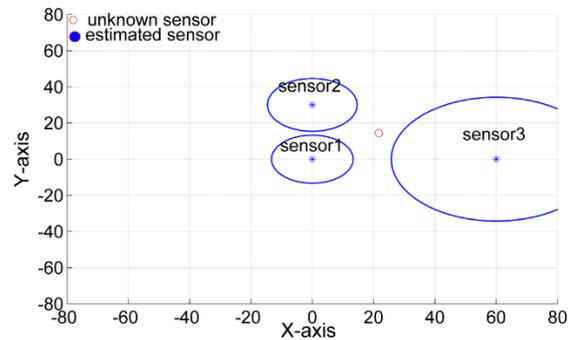
**Figure 10** Estimated sensor (f = 2440 MHz, Po = 4 dBm)
