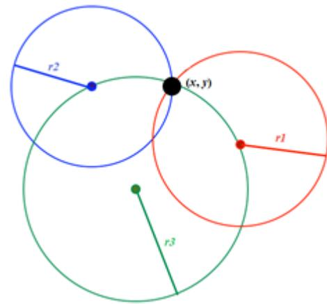
Figure 1 The trilateration algorithm
