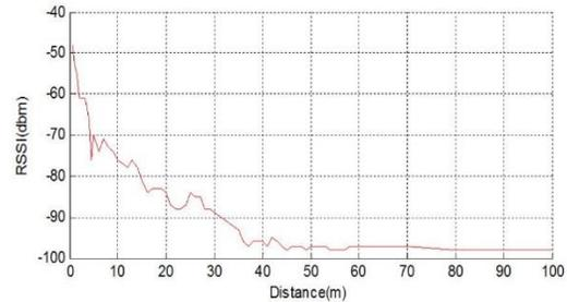
Figure 6 RSSI in function of distance (f = 2440 MHz, Po = -3 dBm)
