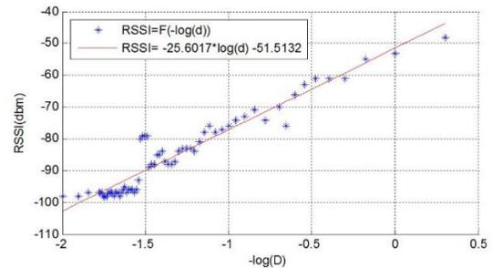
Figure 7 Linearization and interpolation of the measured values of RSSI (f = 2440 MHz, Po = -3 dBm), and the linearization and interpolation of measured values of RSSI allows deducing a model which corresponds to (2).
