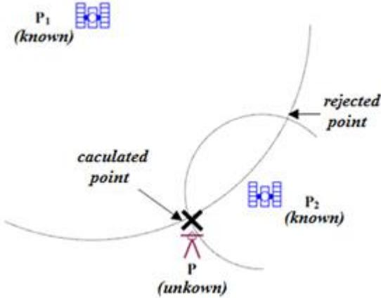
Figure 3 Computing the intersection of the circles
