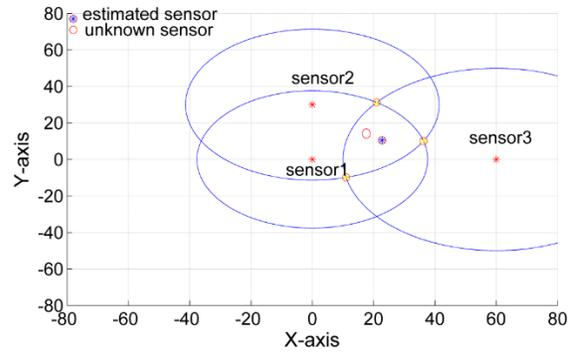
**Figure 8** Estimated sensor (f = 2405 MHz, Po = 4 dBm)
