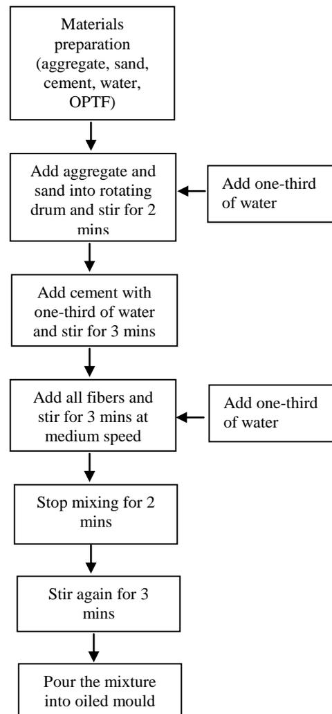
Figure 2: Simplified mixing flow chart
