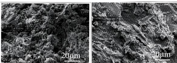
Figure 10: SEM micrograph of concrete after immersion in; (a) NaOH and (b) HCl.
