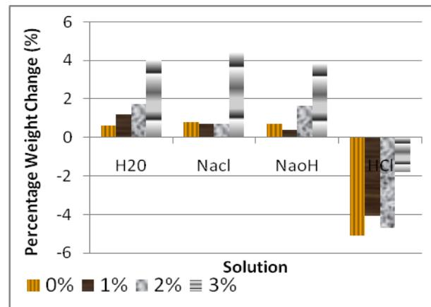
Figure 8: Percentage weight change of OPTF reinforced concrete when immersed in different solution
