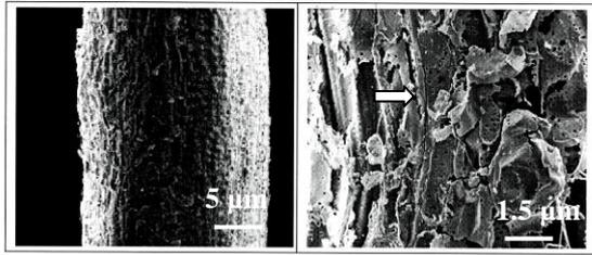
Figure 3: SEM micrograph showing the OPTF fiber at different magnification; (a) 65x and (b) 1500x
