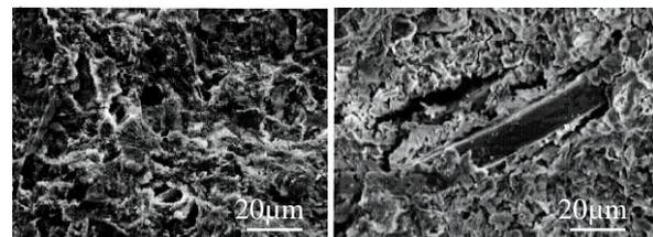
Figure 9: SEM micrograph of concrete; (a) without fiber and (b) with fiber
