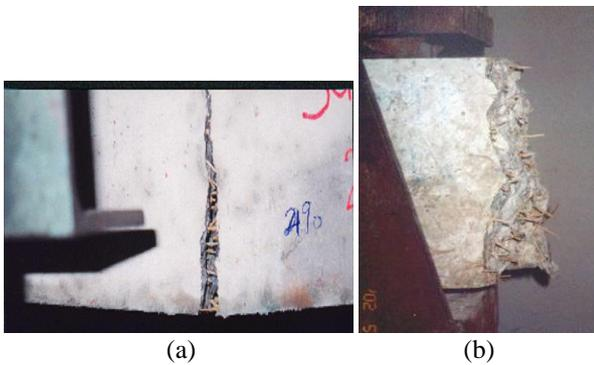
Figure 5: Concrete reinforced with OPTF; (a) specimen under bending showing OPTF as crack arrester and (b) broken specimen showing uniformly distributed OPTF in concrete.
