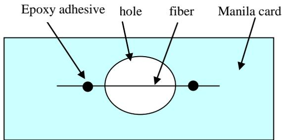
Figure 1: Mounting of fiber for tensile testing on coupon
