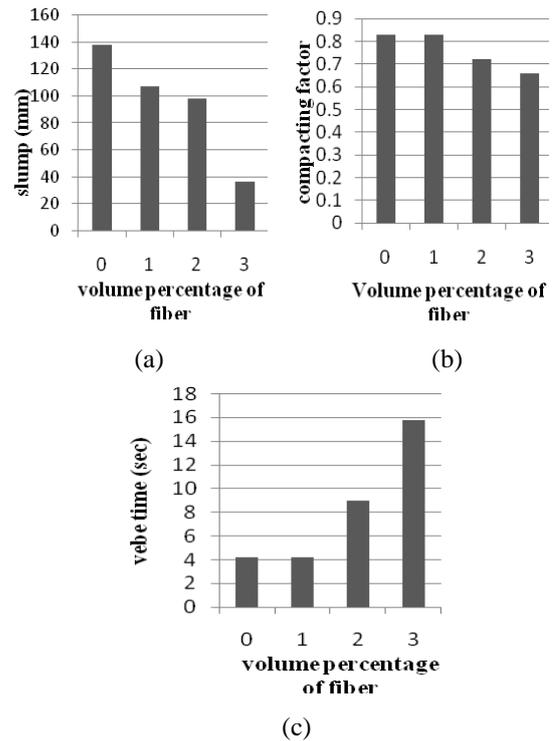
Figure 4: The workability of concrete with different addition percentage of OPTF; (a) slump test, (b) compacting factor and (c) vebe time
