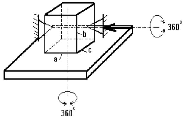
Scheme 1: The principle scheme of the indexing type table.
