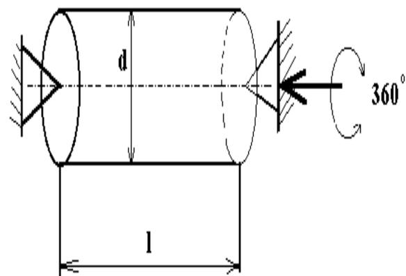
Scheme 2: The principal scheme of the catching and orienting the rotated object.
