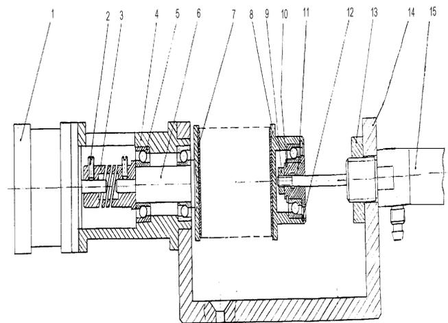
Scheme 4: The orientation and catching subassembly of the piece in the working post.
