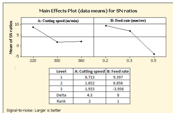
Figure 6 Main effects of parameters in the S/N ratio for tool life
