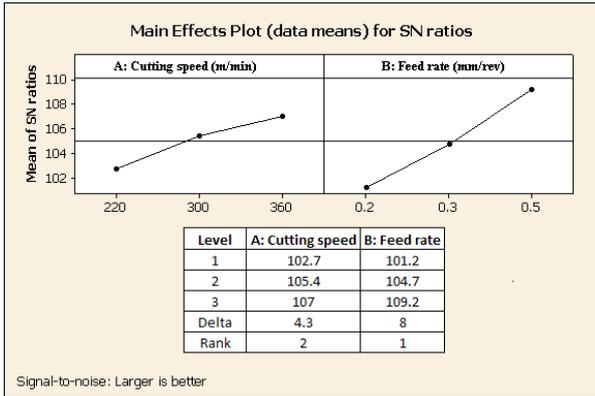
Figure 4 Main effects of cutting speed and feed rate parameters in the S/N ratio for MRR
