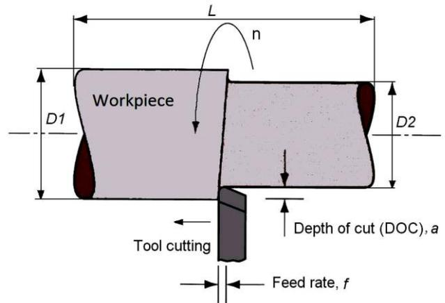
Figure 2 Schematic diagram of the orthogonal metal cutting configuration
