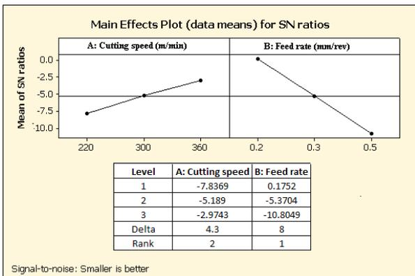
Figure 5 Main effects of cutting speed and feed rate parameters in the S/N ratio for surface roughness
