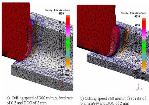
Figure 7 The comparison of total velocity between cutting speed of 300 m/min and 360 m/min (the same feed rate of 0.2 mm/rev and DOC of 2 mm)
