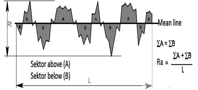
Figure 3 Schematic of parameter definition used to compute the mean arithmetic deviation ( $Ra$ ) and total roughness ( $Rt$ )
