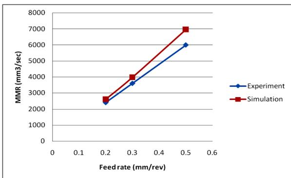
Figure 10 Feed rate vs MRR (feed rate of 0.2; 0.3 and 0.5 mm/rev, cutting speed kept constant at 360 m/min)
