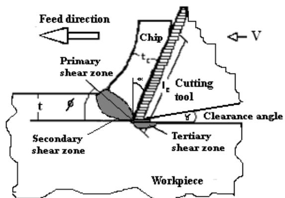
Figure 1 Generation of heat in orthogonal
