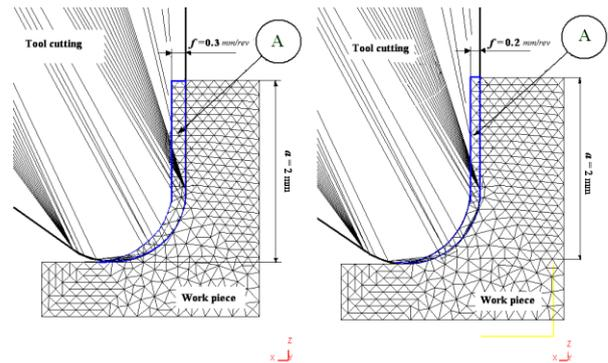
Figure 8 Comparison of meshed geometries between feed rate of 0.3 mm/rev and 0.2 mm/rev (the same cutting speed of 220 and DOC of 2 mm)
