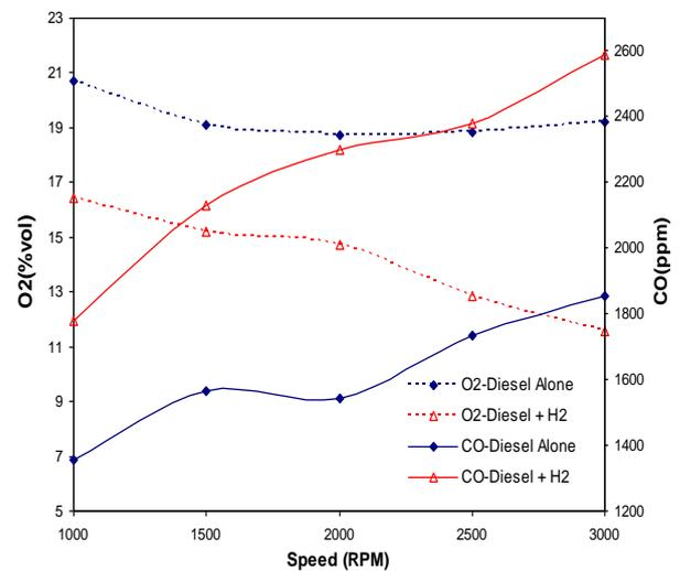
Figure 6 Variation of O<sub>2</sub> and CO emissions with engine speed
