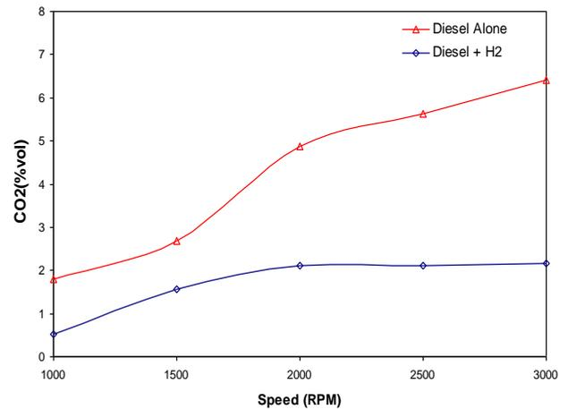
Figure 5 Variation of CO<sub>2</sub> emissions with engine speed
