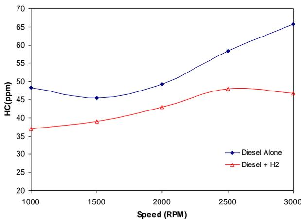
Figure 4 Variation of HC emissions with engine speed
