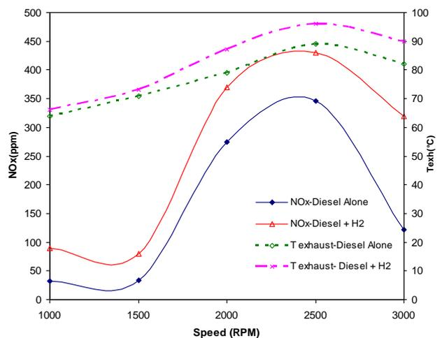
Figure 3 Variation of NO<sub>x</sub> emissions and exhaust gas temperature with engine speed
