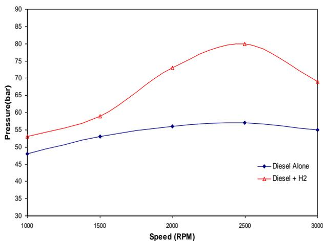
Figure 2 Variation of in-cylinder peak pressure with engine speed
