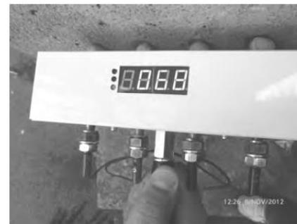
**Figure 12** ERT measurement apparatus called ASMR [20]
