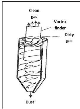
Figure 1 Cyclone with axial entry [4]
