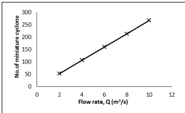
**Figure 6** Number of miniature cyclones in MR-deDuster for different flue gas volumetric flow rates
