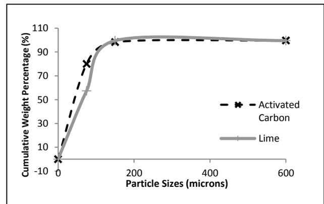
**Figure 4** Particle size distribution of adsorbent materials [17]
