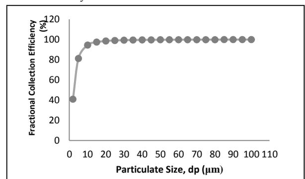
**Figure 5** Fractional collection efficiency prediction of MR-deDuster on activated carbon dusts particles
