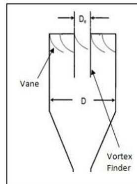
Figure 3 Schematic diagram of a miniature cyclone [15]
