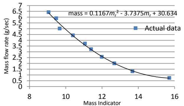
Figure 3 Mass flow rate measurement using the direct method [18]
