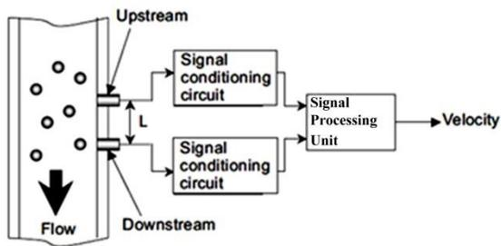
**Figure 4** Block diagram of velocity measurement using the cross-correlation technique [6]
