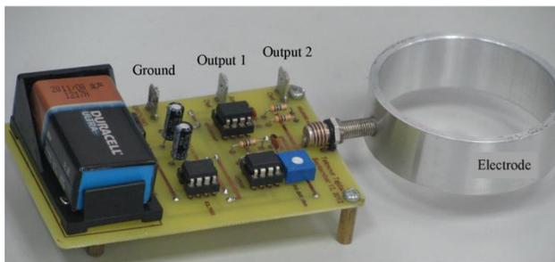
Figure 2 A typical electrostatic sensor [9]
