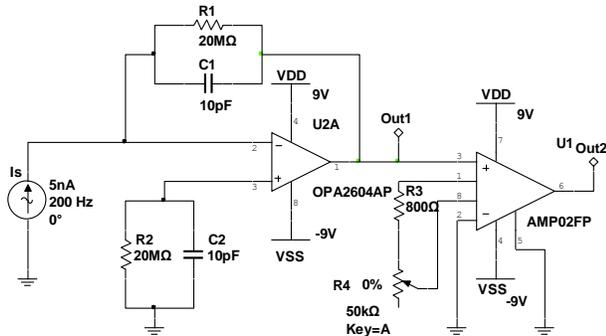
Figure 1 A typical electrostatic signal conditioning circuit [9]
