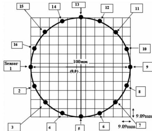
**Figure 5** Sensor arrangement for 11x11 rectangular array maps on a cross section pipe [41]
