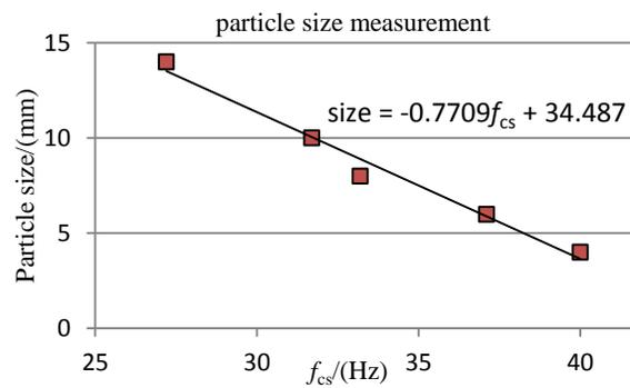
Figure 6 Particle size measurement results with frequency
