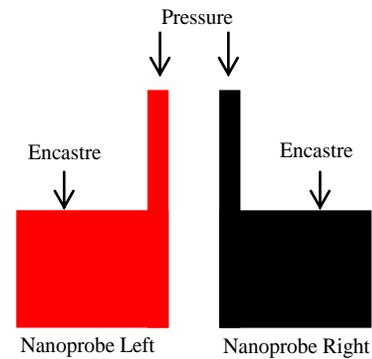
**Figure 5** Simulation setup for the dual Nano probe's mechanical characterization
