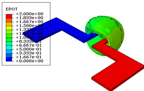
Figure 11 Electrical potential distribution when applying 2 Volts
