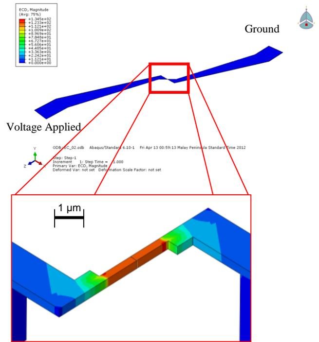
Figure 7 Current density on the dual nanoprobe. Inset image shows the magnified view of the dual nanoprobe
