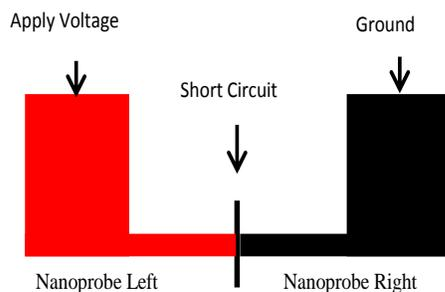
**Figure 4** Simulation setup for the dual Nano probe's electrical characterization
