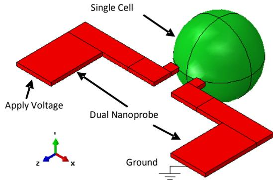
Figure 6 Simulation setup for the single cell electrical measurement
