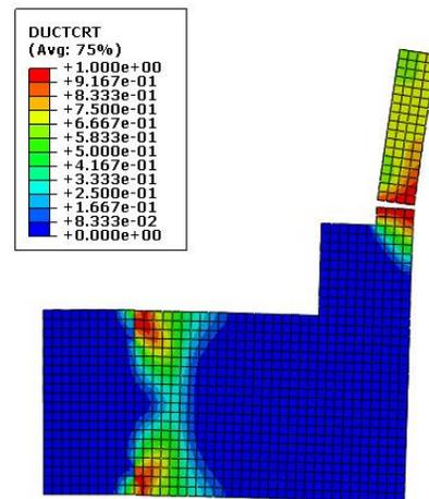
**Figure 9** Nano probe damage simulation
