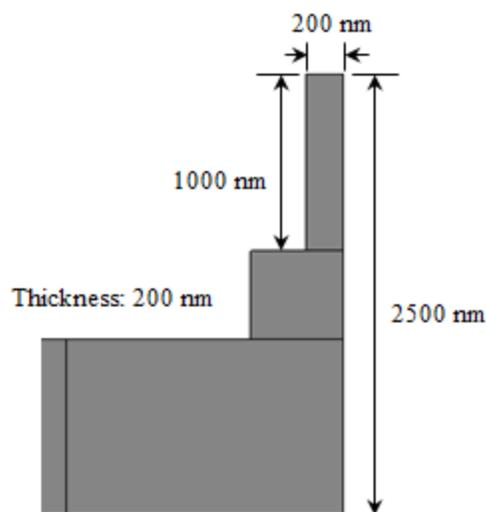
Figure 3 Nano probe dimension
