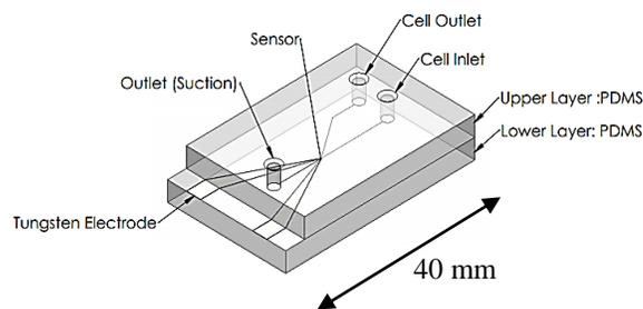
Figure 2 Dual Nano probe-microfluidic integrated system
