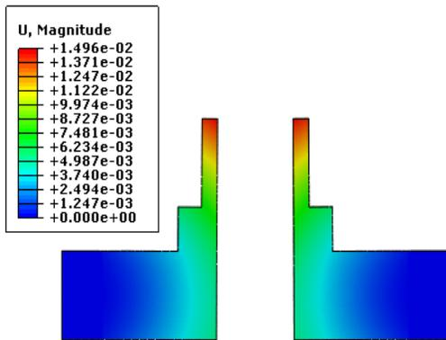
**Figure 8** Displacement of the dual nanoprobe
