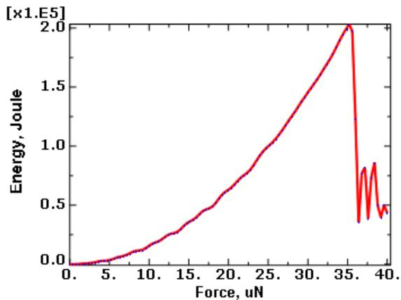
Figure 10 Strain energy of Tungsten Nano probe
