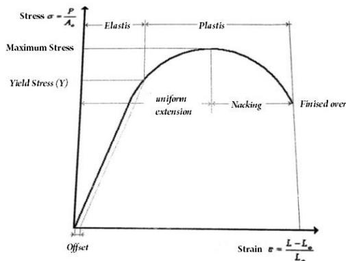
Figure 2 Graph stress versus strain
