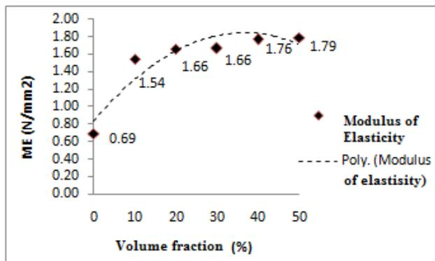
**Figure 8** Graph showing the relationship between the modulus of elasticity (E) with a ratio of volume fraction variation
