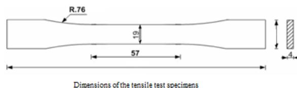
Figure 4 Dimensions of tensile test specimens standard ASTM D638-10
