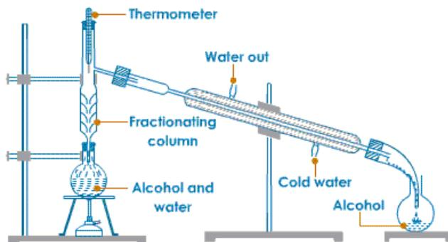
Figure 3 Fractional distillation process [9]
