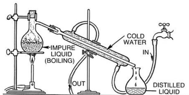
Figure 2 A typical distillation process [8]
