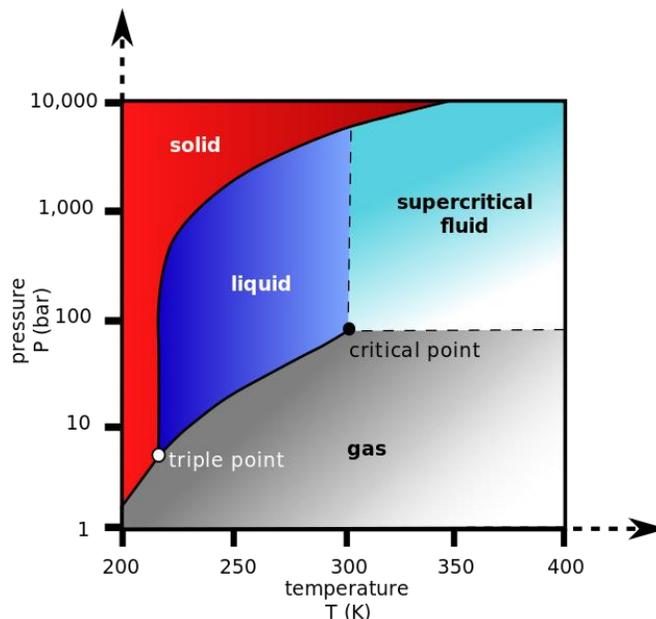
Figure 1 Phase diagram for carbon dioxide [6]
