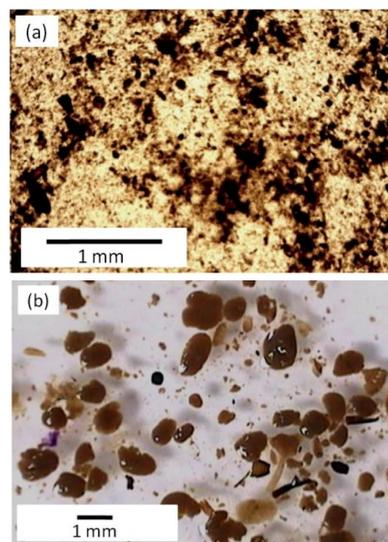
**Figure 1** Morphology of AGS in the reactor (a) Fluffy and filamentous aerobic granular sludge at 14<sup>th</sup> day of inoculation (b) Matured and dense aerobic granular sludge at day 60 of inoculation
