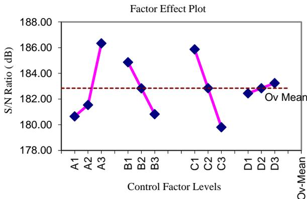
Figure 4 Factor effect plot for SNR (Smaller-the-Better)
