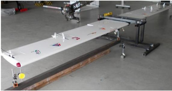
Figure 5 Wing-to-rig attachment
