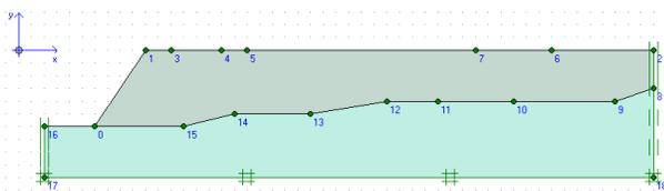
Figure 6 Plaxis 7.2 model for fill and slope<sup>1</sup>
