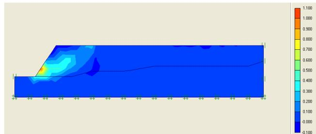
Figure 9 Incremental strains after heavy rain<sup>1</sup>
