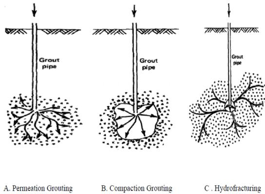
Figure 5 Types of grouting system<sup>6</sup>
