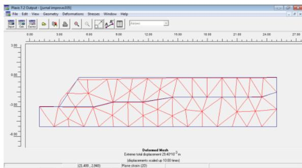
Figure 10 Deformation after cement grouting<sup>1</sup>
