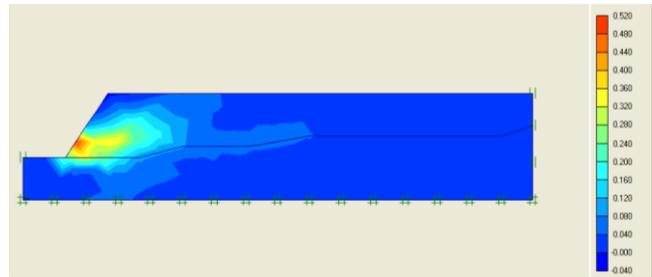
Figure 7 Strain in the slope when soil is dry<sup>1</sup>
