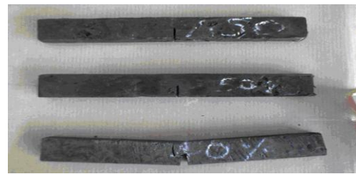
Figure 6 SENB specimens of C/C composites
