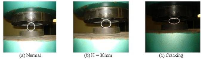
Figure 3 Flattening test
