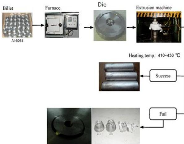
Figure 1 Processing of hot extrusion of Al 6061 alloy tubes using porthole-die
