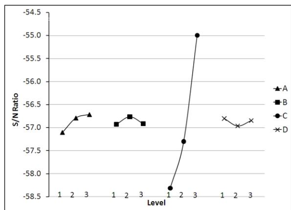
Figure 4 Main effects of control factors on Extrusion load
