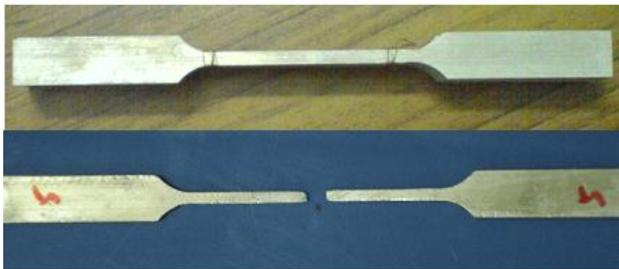
Figure 2 Failure of test piece during tensile test
