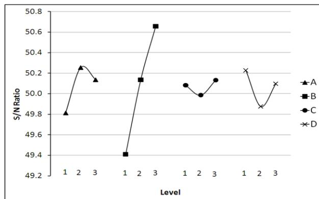
Figure 5 Main effects of control factors on Tensile strength
